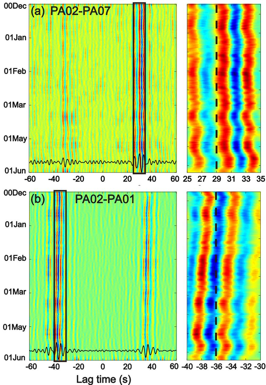
**Figure 3.** Noise cross-correlation functions (NCCF) from hydrophone recordings at two OBS pairs, with colour indicating the amplitudes of the NCCF. (a) Very little change in arrival time of the largest amplitude, whose zoom-in window is shown in the right-hand panel. Black trace is the stacked NCCF over all days. (b) Clear time drifting indicated by the change of the NCCF between PA02 and PA01 stations.
