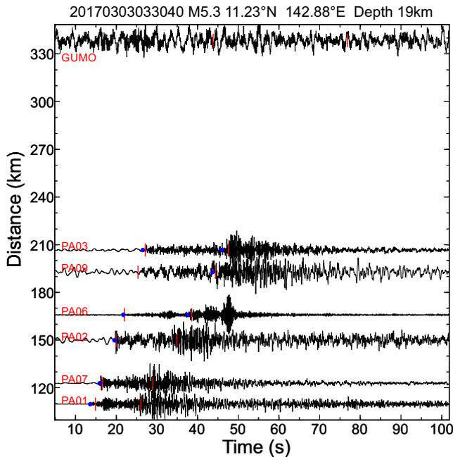
**Figure 11.** Waveforms of a  $M5.3$  earthquake (location shown as the red star in Fig. 9a) that is missed in the USGS catalogue due to a lack of impulsive arrivals at GUMO. Red bars and blue dots indicate the theoretical and hand-picked arrival times of  $P$  and  $S$  waves, respectively.
