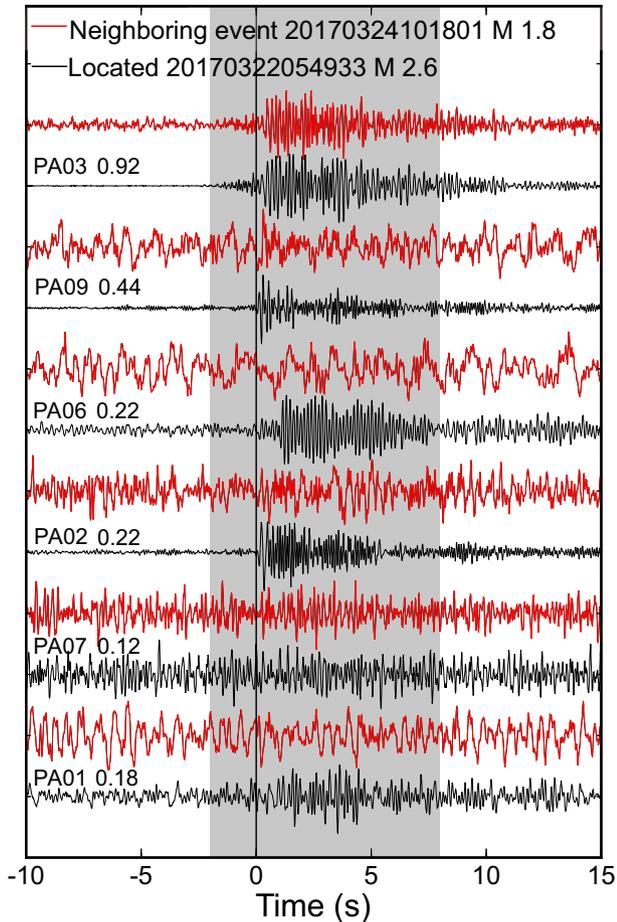
**Figure 7.** Waveforms of an earthquake located using Hypoinverse (black) and a detected, neighboring earthquake (red) aligned by  $S$ -wave arrivals. The grey shadow marks the time window (2 s before and 8 s after the  $S$ -wave arrival) used for waveform cross-correlation. The station names and cross-correlation coefficients are marked on the left.
