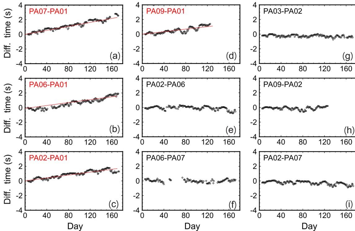
**Figure 4.** Temporal variation of relative clock errors between each OBS pair determined by the changes in the largest amplitude of the NCCF. (a–d) Obvious linear time drifting between PA01 and other OBSs. Red lines show the best-fitting linear trend. (e–i) Subtle time drifting among PA02, PA03, PA06, PA07 and PA09 OBSs.
