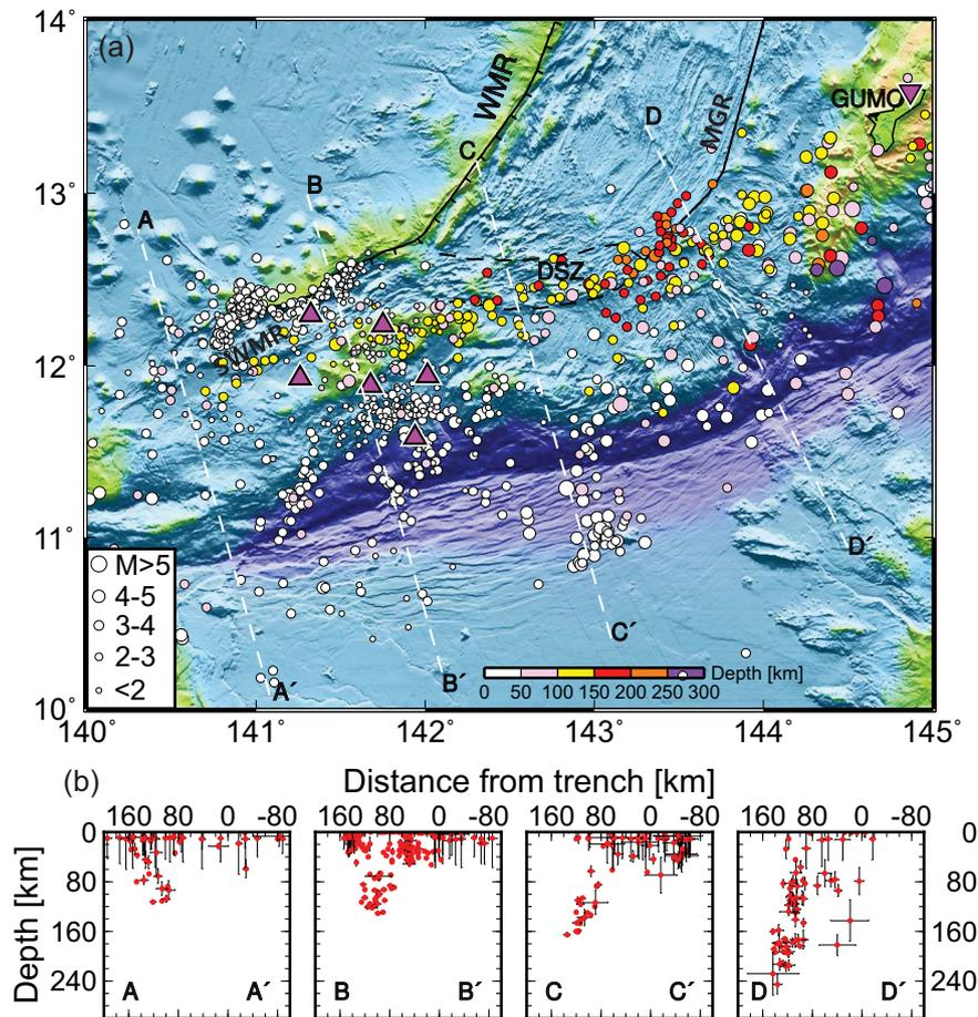
**Figure 6.** (a) Map of absolute earthquake locations (circles) coloured by depth based on the first OBS (triangles) observation in the southern Mariana subduction zone. (b) Cross-section view with a bin width of 30 km of seismicity (red dots) with locations shown panel (a). The horizontal and vertical black bars represent horizontal and vertical location uncertainties, respectively. Trench locations are marked as 0 km.
