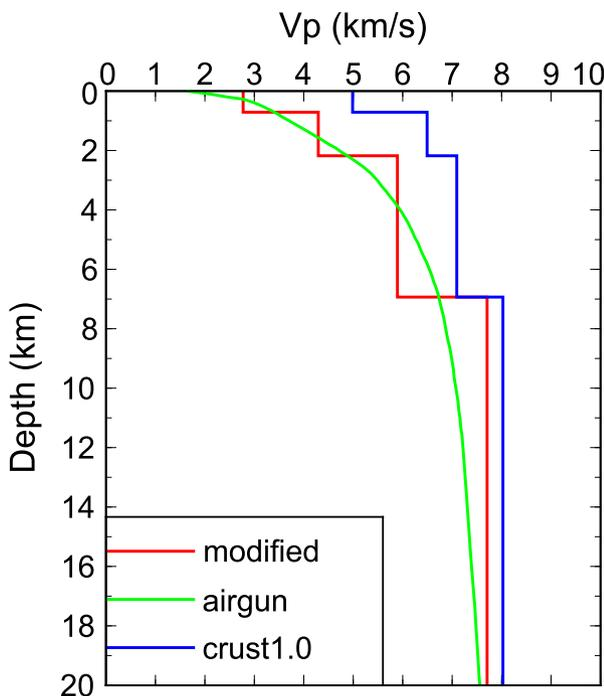
**Figure 5.** The blue line denotes the Crust 1.0 velocity model in the region. The green curve shows the average new  $P$ -wave velocity derived from multi-channel seismic reflection experiment (Wan *et al.* 2019). The red is modified based on the two and is used in earthquake location.
