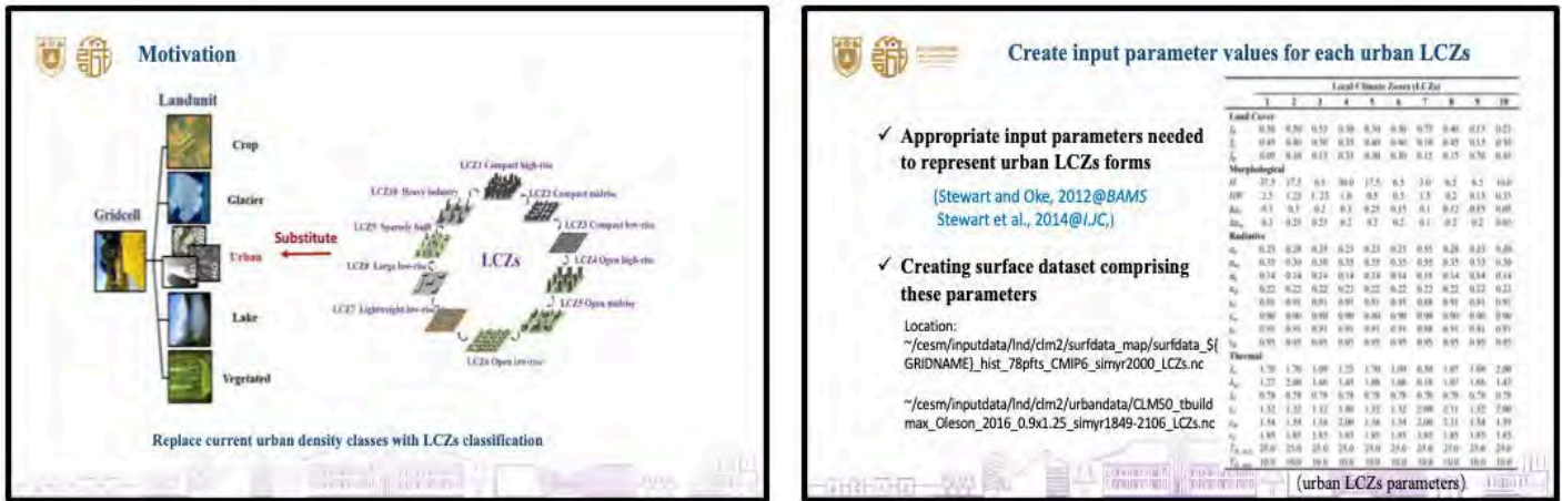
Figure 4. Implementing UCPs from LCZ into the UCLM land use processor (UCLM5) of the CESM.
