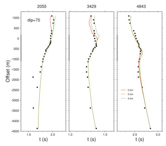
Figure 11. Observed (dots) and model-predicted *P* arrival times (lines) for event 2055, event 3429 and event 4843 for a 70°-dip LVZ. Colours correspond to different LVZ depths.
