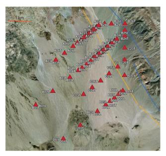
**Figure 2.** Red triangles stand for the temporary array. Two segments of the Calico fault are shown near the array. Orange indicates Holocene faults and blue is Quaternary (U.S. Geological Survey & California Geological Survey 2006).
