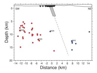
**Figure 8.** A cross-section view of event locations (colour dots) and stations (triangles). Blue and red colours represent positive and negative *P*-wave traveltime differences between the northeastern most and southwestern most stations of the B array, respectively. Grey bar shows the dip and depth of the low-velocity zone obtained in this study.
